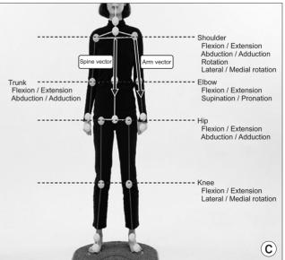
Figure 1. (A) Kinect-V2 (Microsoft, Seattle, WA, USA; 2014). (B) The location of the depth sensor-based motion analysis system was installed at a distance of 1.5 m to the ground, and the distance to the patient was fixed at 2 m. (C) In order to measure the angle of the shoulder joint, a spinal vector connecting the center of the cervical joint and the hip joint was used, and the angle between the spine vector and the arm vector was measured.
